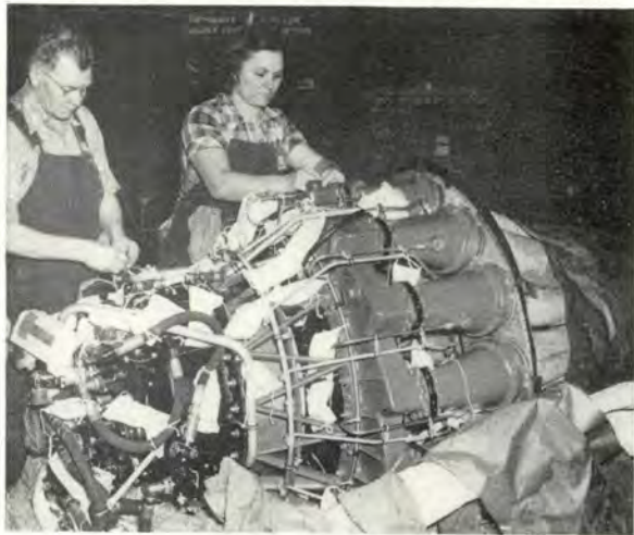
Below. J-33 engines being prepared for storage. Bags contain silica jell. Engine is final-wrapped in heavy metal-foil paper.
