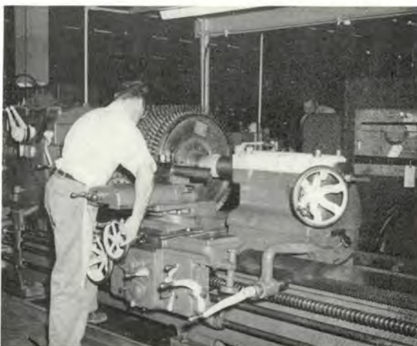
Below. J-35 compressor rotor is machined to correct diameter in the "Parts Rework" section of jet engine overhaul.
