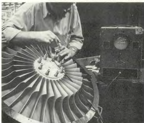
Below. J-35 compressor rotor is machined to correct diameter in the "Parts Rework" section of jet engine overhaul.
